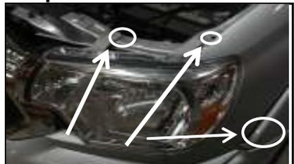
Remove 2 bolts located on top of the headlight and 1 bolt located
