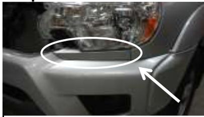
Remove the plastic piece carefully by unclipping it and pulling it towards the grill located
